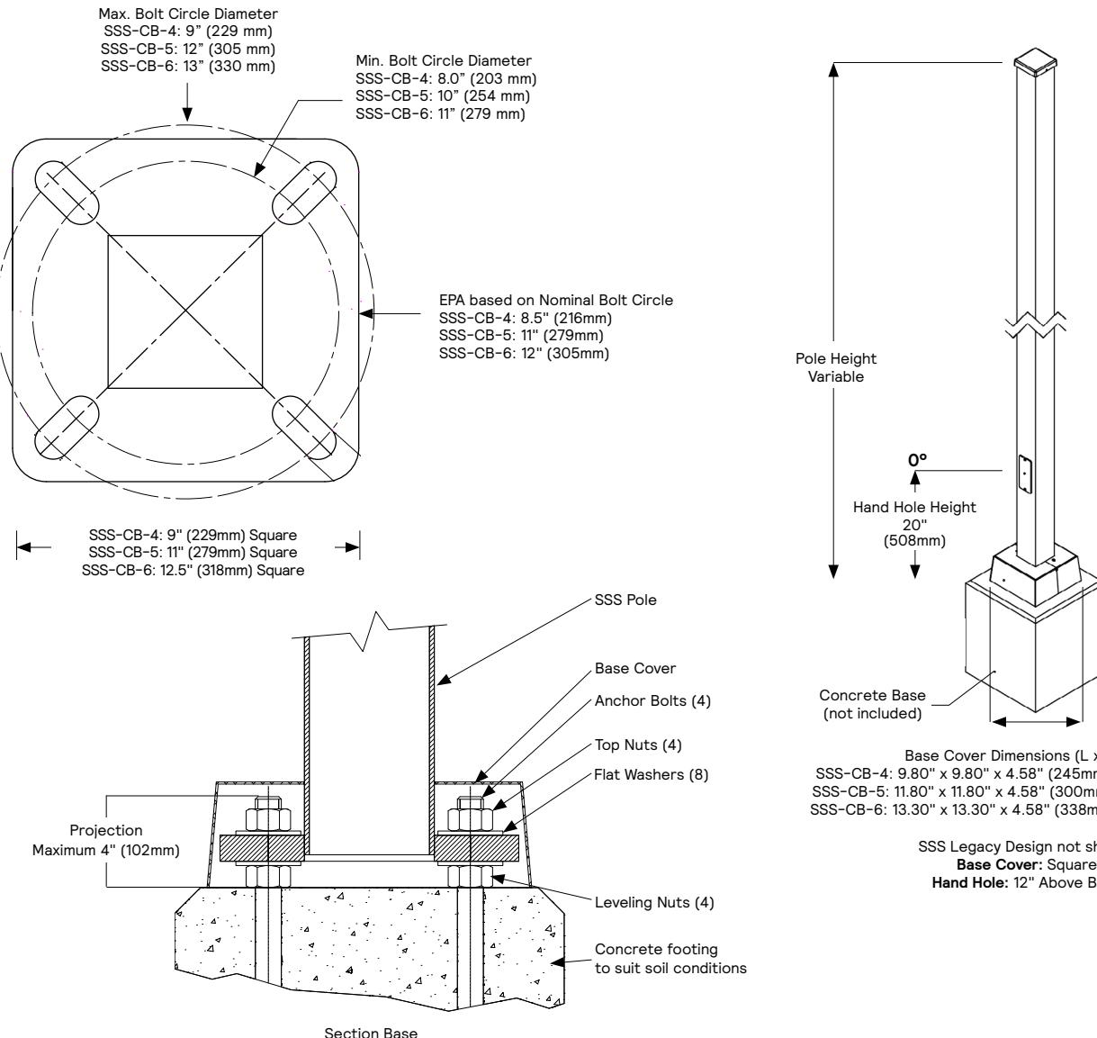
\* Anchor Bolt Lock Washers are not normally required and are not included in standard anchor bolt sets. They are available upon request at additional cost.
